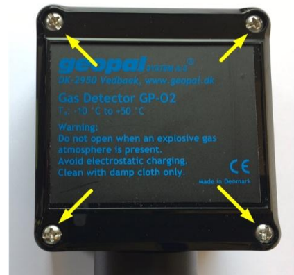
Figure 1: Front cover with the four screws indicated by the yellow arrows.
