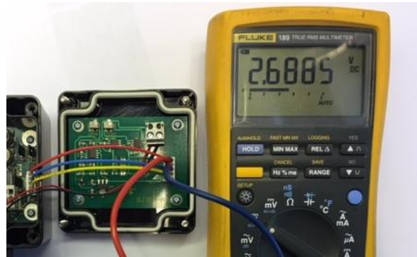
Figure 4: Typical output voltage value of 2.7 V when the detector is exposed to atmospheric air.
